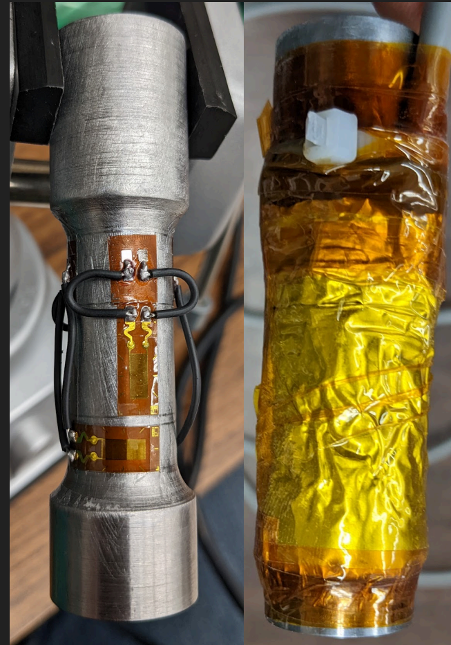
Impact Force Load Cell
